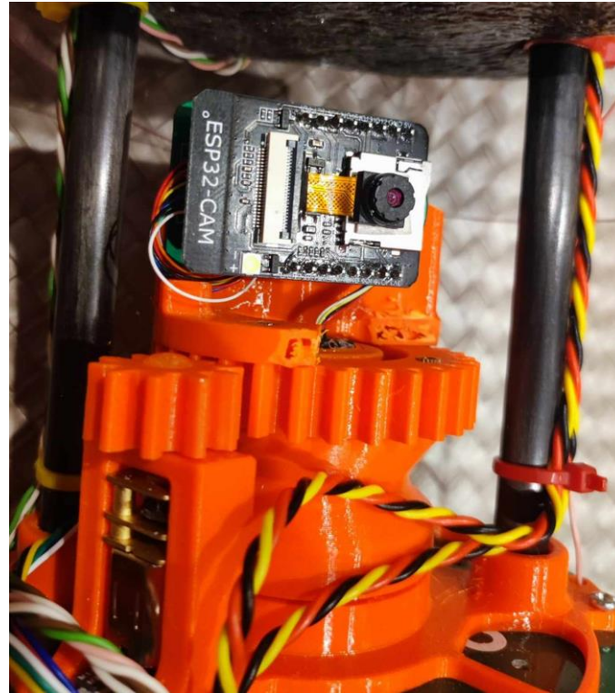
Camera stabilization mechanism
